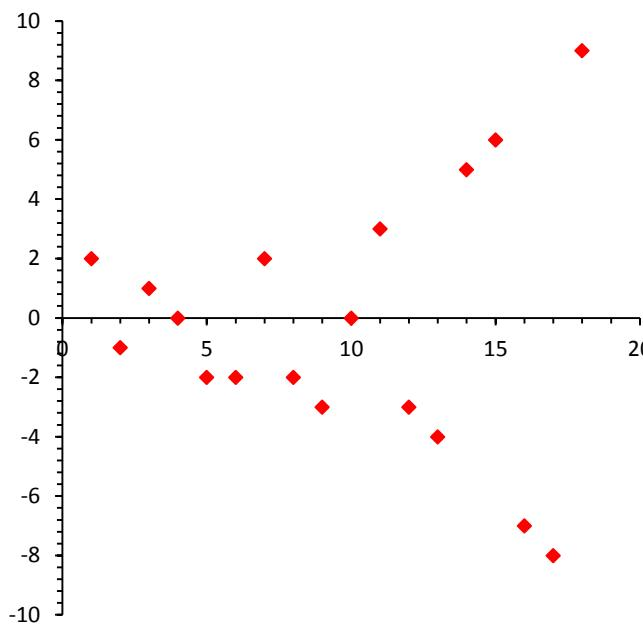
The U-shaped residuals plot is the result of fitting a straight line to data which are better represented by a curve. There is a lack of fit with the straight line model
