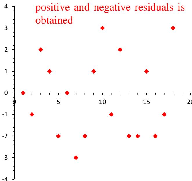
the condition of homoscedasticity is not fulfilled: the scatter of the residuals increases with y. This indicates that the precision of the measurements over the concentration range considered is not constant
