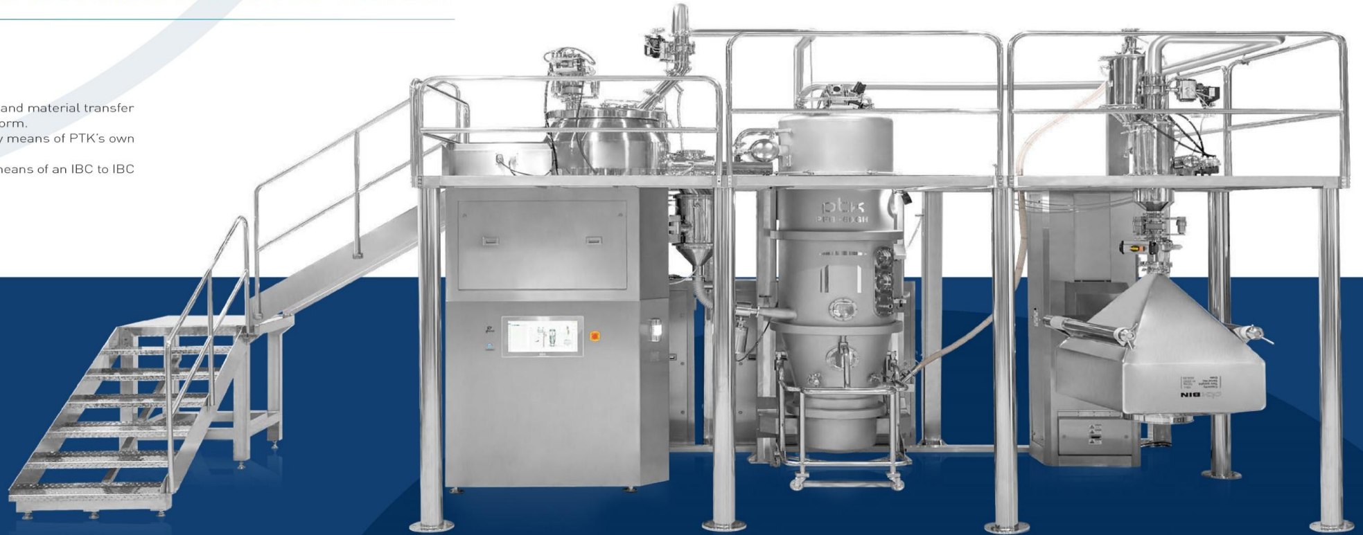
Integrated computer control of the entire granulation line.
